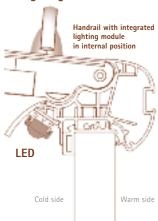
LED lights on the inside of the handrail could be completed in addition with LED fixed on the push sliding profile. LED lights enable lower energy consumption and an increased life cycle.
