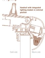
Fluorescent tubes operate better in a warm environment outside of the combust. Most of the harmful thermal infrared radiation is reflected through the insulating glass on the side.
