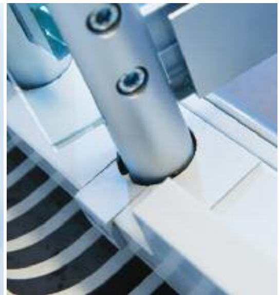
covered protection of the door draw system
